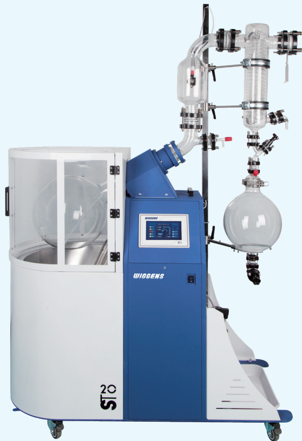
Vertical glassware (Vapor sinking)
