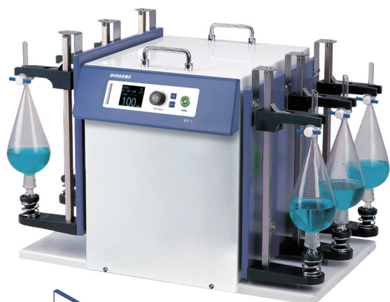
WS-1 Angle is not adjustable
